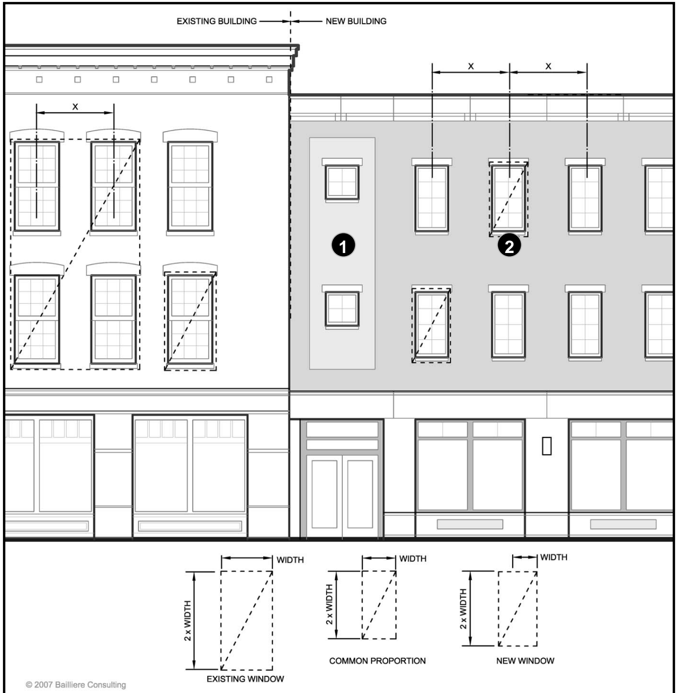
Figure 5 (above): Examples of common proportions on two different buildings. Although the building on the right has smaller sized windows than the older building on the left, they share similar proportions to each other which helps to visually tie the two facades together. Both sets of windows are approximately twice (2x) as tall as they are wide. The spacing of windows has a similar rhythm which also helps to give the different designs a common theme.
