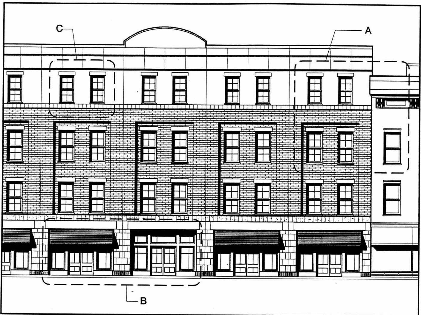
Figure 10: Shadows on elevation show depth in facade.
