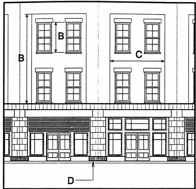
Figure 7: Vertical proportions in a facade.
