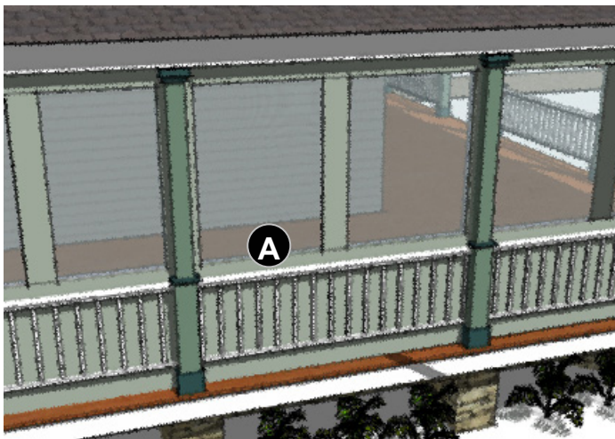
Fig. 1: Although it is not recommended that existing porches be enclosed or converted to screened porches, if it is done the new enclosure should incorporate the original porch construction as shown above so that it remains exposed as a relief on the new enclosure.
